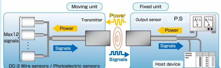
An output sensor in fixed unit connects a power supply and external control devices such as a PLC. A transmitter in moving unit connects detection sensors.
