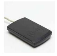
ID Reader/Writer writes to the ID tag by USB or RS-232C connecting to the PC.
